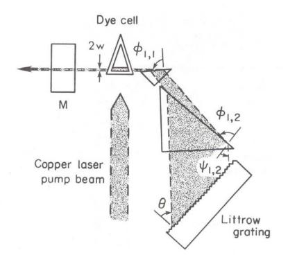
Fig.1. CVL-pumped narrow-linewidth multiple-prism grating tunable laser oscillator. In this closed-cavity dispersive oscillator configuration the beam waist at the gain medium (*w*) is reduced to achieve single-transverse-mode emission. The resulting beam dimension (2*w*) is then expanded to completely illuminate the diffraction grating. For this particular oscillator the beam magnification factors is  $M \approx 100$  (from Duarte and Piper (10)).
